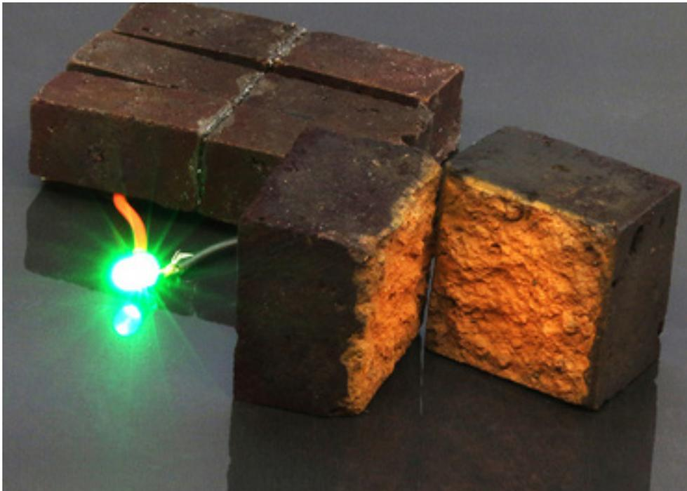
Chemists in Arts & Sciences have developed a method to make or modify "smart bricks" that can store energy until required for powering devices. (Image: D'Arcy laboratory)
