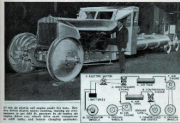
27 lbs. air electric cell engine ready for use. Battery drive electric motor running, heating air compressed to 400 lb. pressure by air motor on motor drive and electric drive main compressor in 100 tanks, and burner charging generator.
